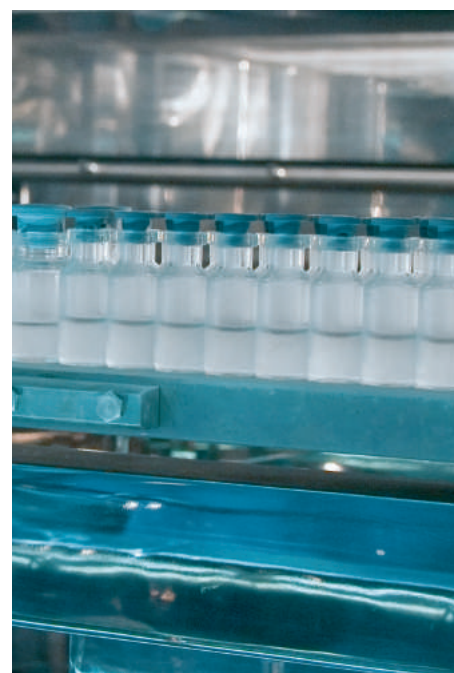
After ice fog injection/all vials nucleated
