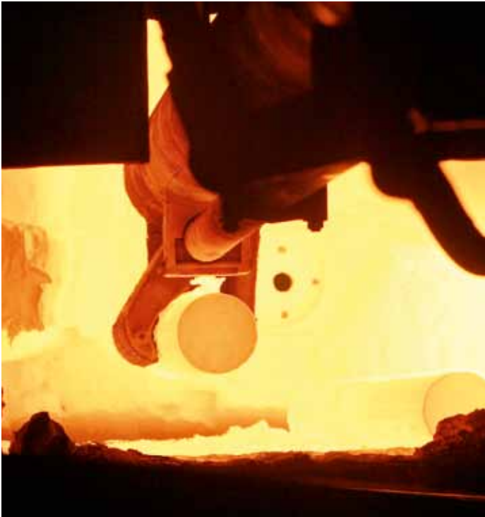
Extraction of reheated material from a furnace using REBOX® technology
