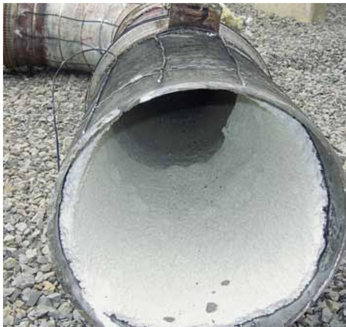
Figure 32: Ammonia salt deposits in a pipe
