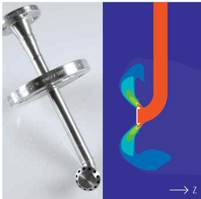
Figure 15: OXYMIX Injector for oxygen enrichment. Photograph (left) and flow pattern (right) of oxygen being fed into the process air pipe
