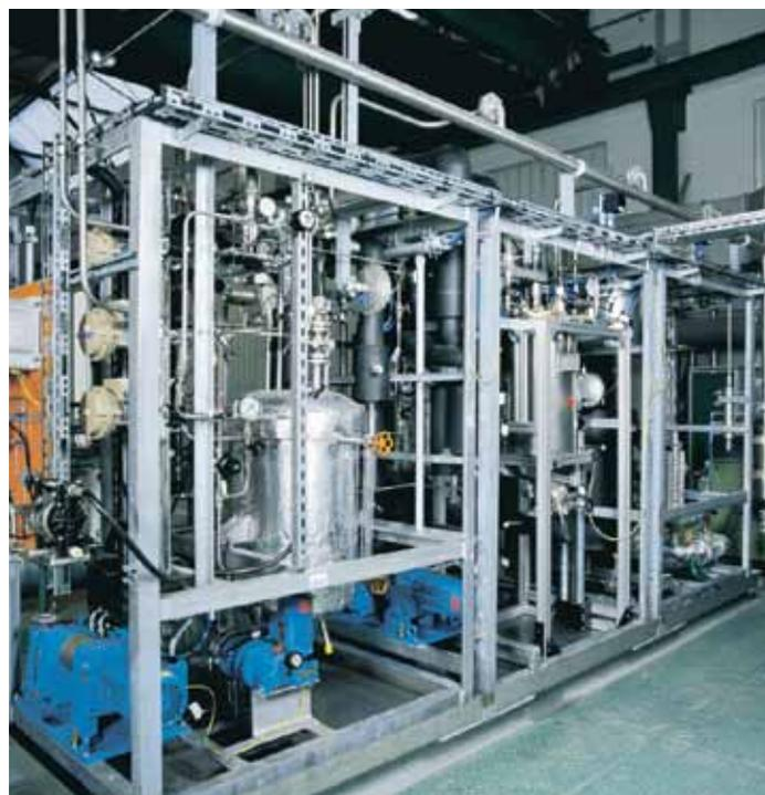
Figure 46: The stirred tank reactor test system
