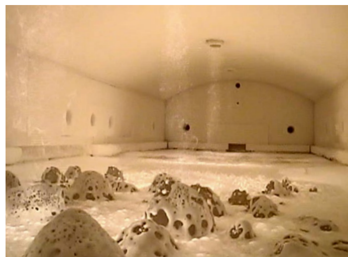
COROX® convective glass melting in operation
