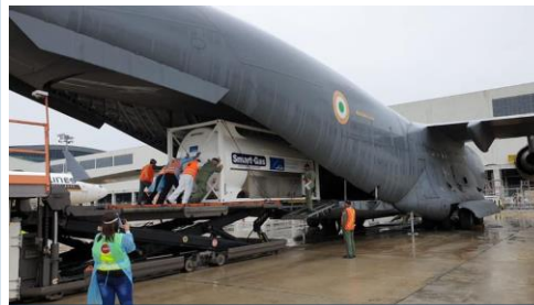
Indian Air Force C-17 Globemaster III aircraft carrying 4 x 20T ISO Tanks from Singapore
