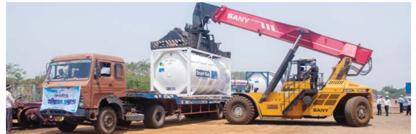
ISO Cryogenic containers airlifted from overseas, which can carry up to 20 tons of Liquid Oxygen over long distances.
