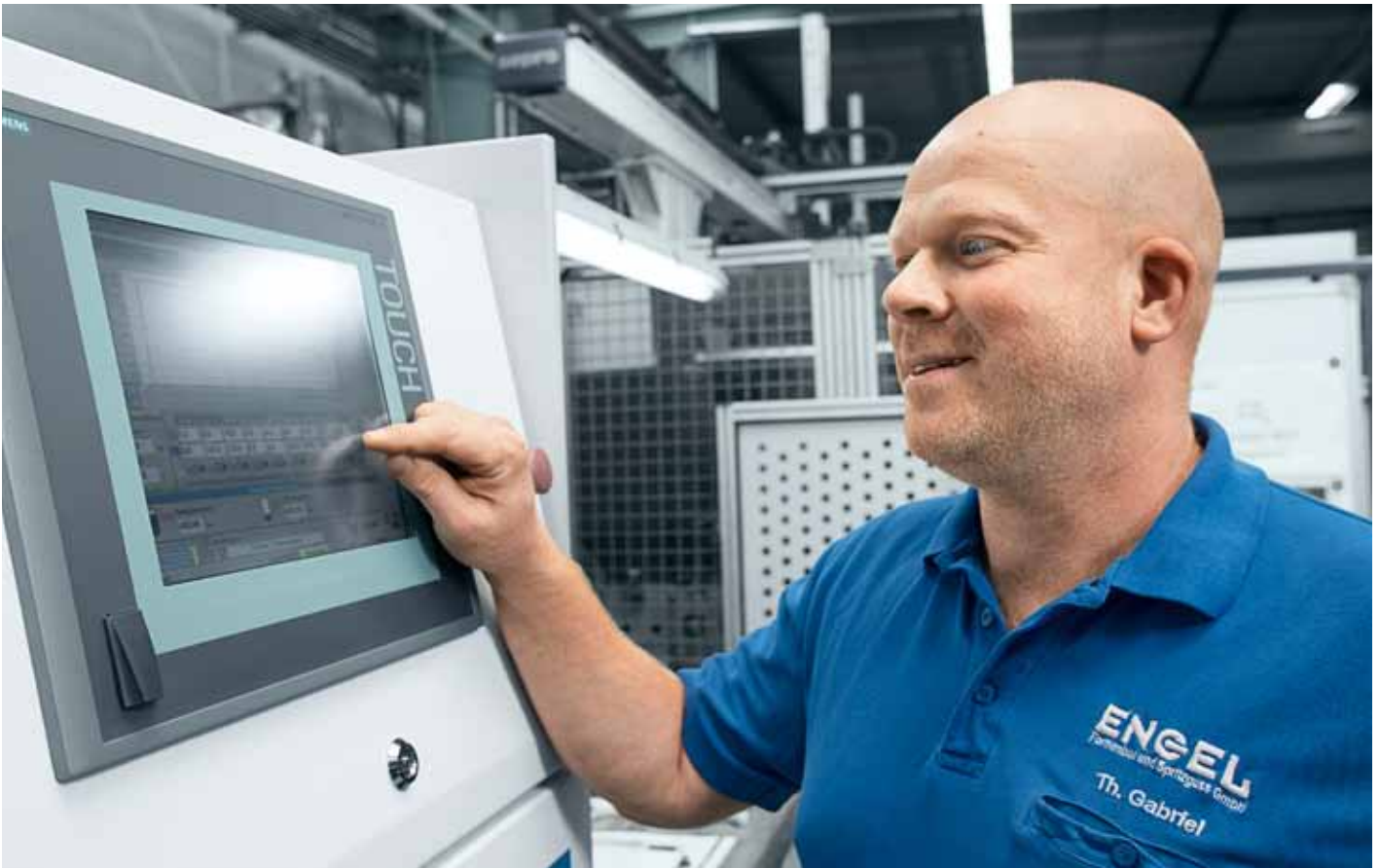
The CO 2 pressure control unit offers an intuitive user interface for adjusting process parameters.
