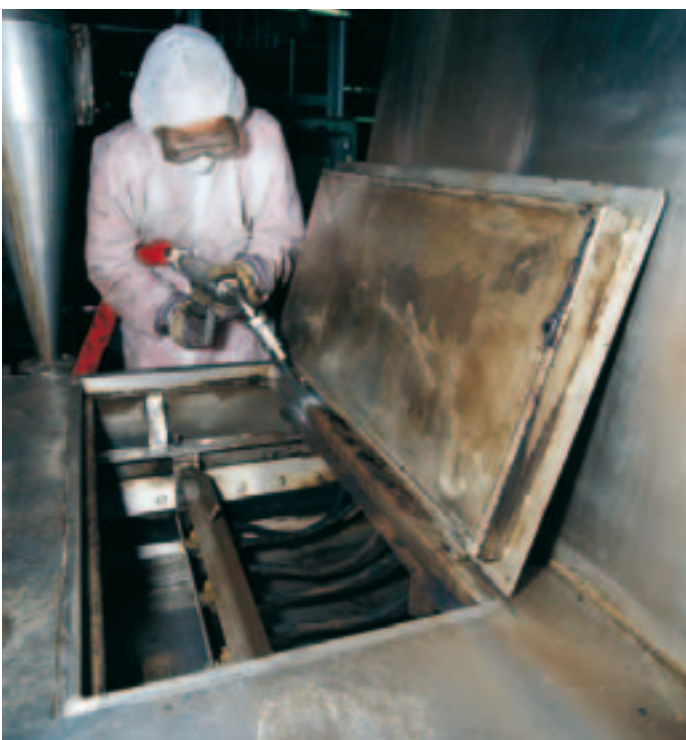
Fig. 17: Cleaning with the CRYOCLEAN® process in a coffee processing plant
