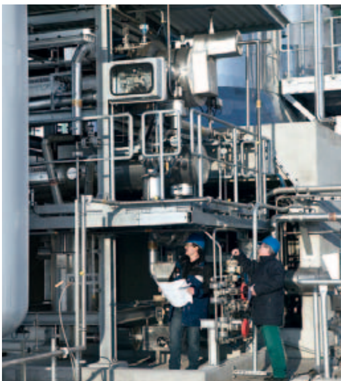
Fig. 13: CRYCON® cryocondensation unit in fine chemistry
