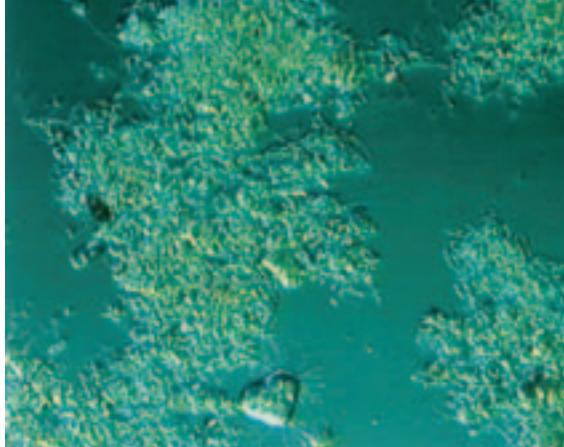
Well-developed sludge flocks after 14 days of oxygen treatment.
