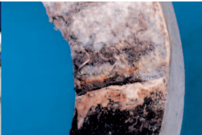
Costly: corrosion damage to a pressure pipe.
