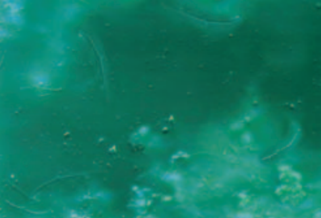
Weakly structured flocks caused by inadequate oxygen supply in the wastewater treatment plant of a brewery.
